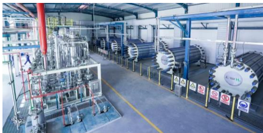
万吨级光伏制氢项目碱性电解水制氢厂房 10000-ton Solar-coupled Alkaline Electrolysis Water Hydrogen Production
